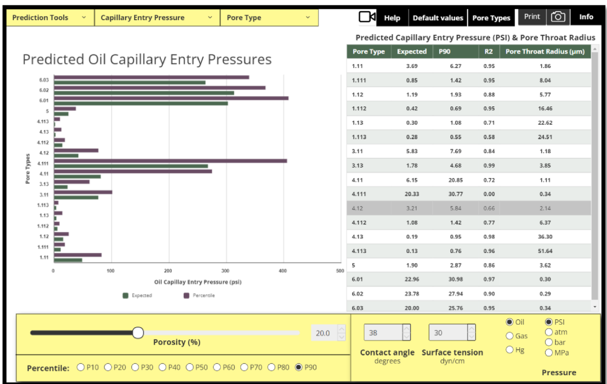
Figure 10 Capillary entry pressure prediction window inside CARP tool (CARP Software).
