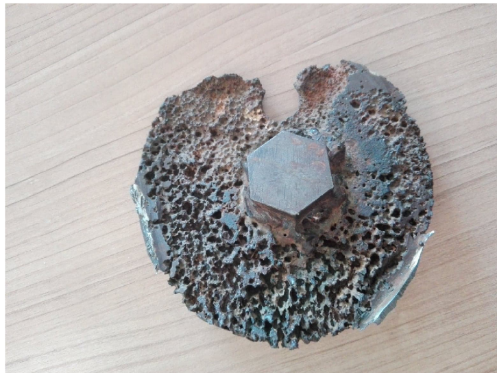
Figure 1.1: Component severely damaged by cavitation. (photograph courtesy of Dr. Pavel Rudolf).
