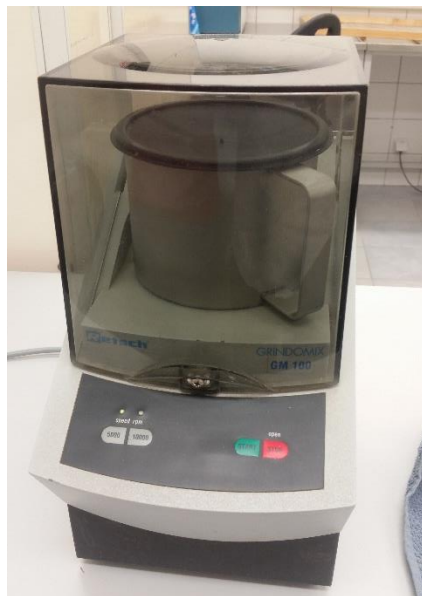
Figure 4.3 Retsch Grindomix GM 100 Grinding knife mill
