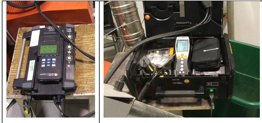
Figure 4.23 Devices for combustion analysis: Testo 350 (left), Testo 380 (right) Source: Research Institute of Agricultural Engineering, 2017.
