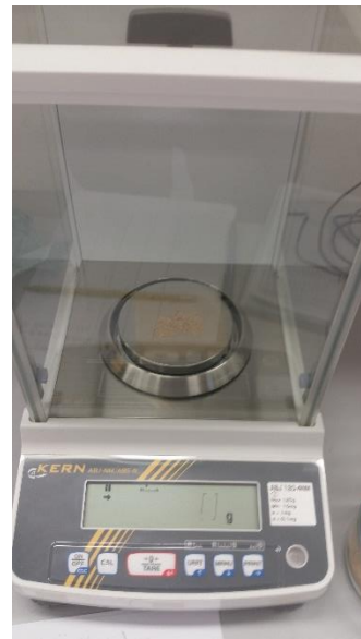
Figure 4.5 KERN laboratory scale (model ABJ 120-4NM) Source: Author, 2017
