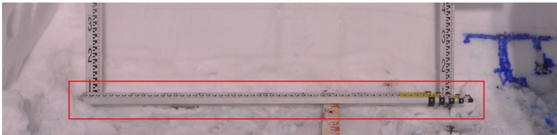
Figure 29: Bottom scale facing upwards causing laborious consequences at determining the horizontal accumulation of water. Photo by supervisor of this thesis
