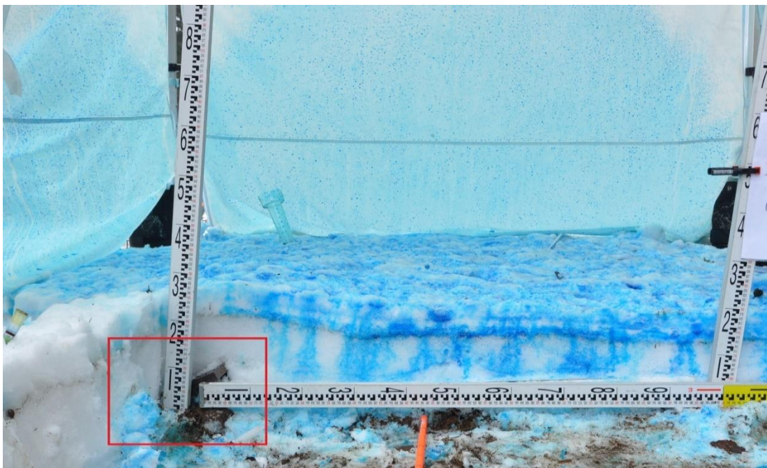
Figure 30: An example of disconnected scales causing difficulties in horizontal water accumulation determination. Photo by supervisor of this thesis
