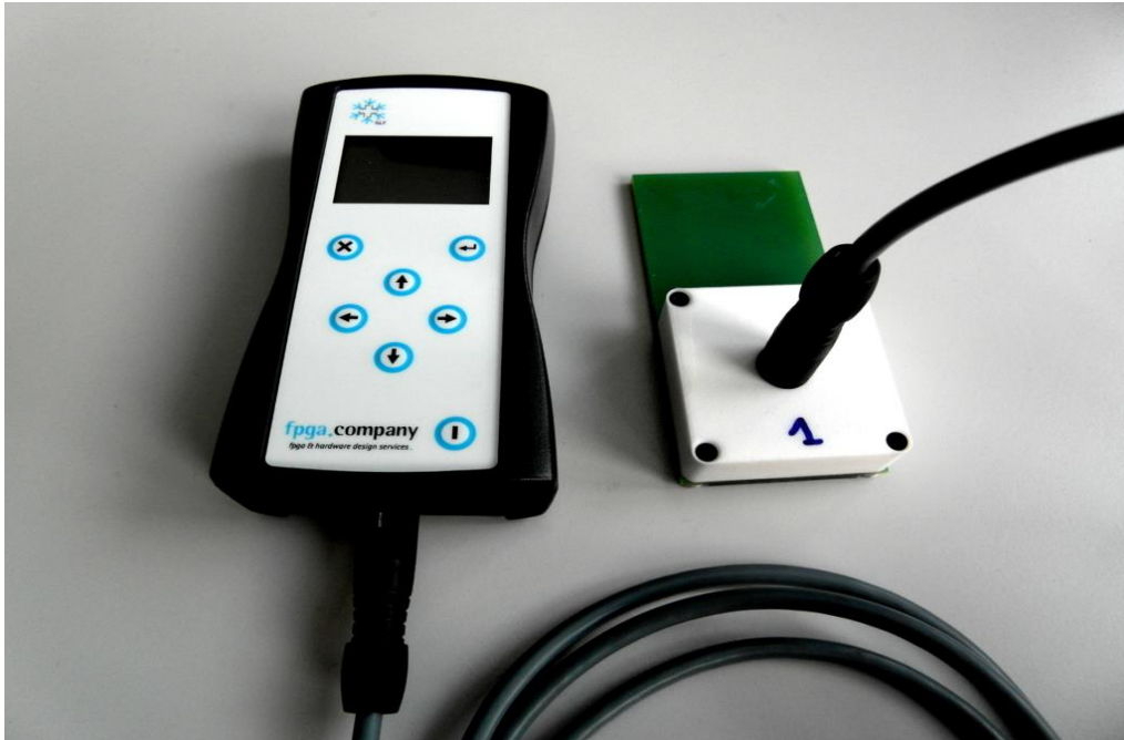
Figure 8: The SLF Snow Sensor based on the Denoth Meter capable of measuring density of snow and liquid water content. Adapted online from FPGA COMPANY © (2020)
