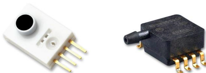
Obr. 7.8: Senzory tlaku Freescale: zleva MPX2300DT1 a MPXV2053GP [16, 17]
