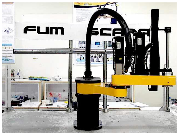
Obr. 19: FUM SCARA robot [33].
