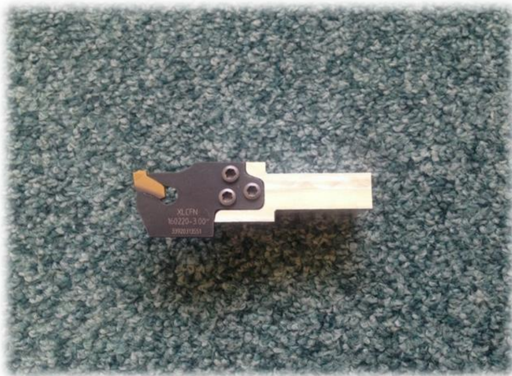
Figure 6.41: New CNC tool holder with the tool
