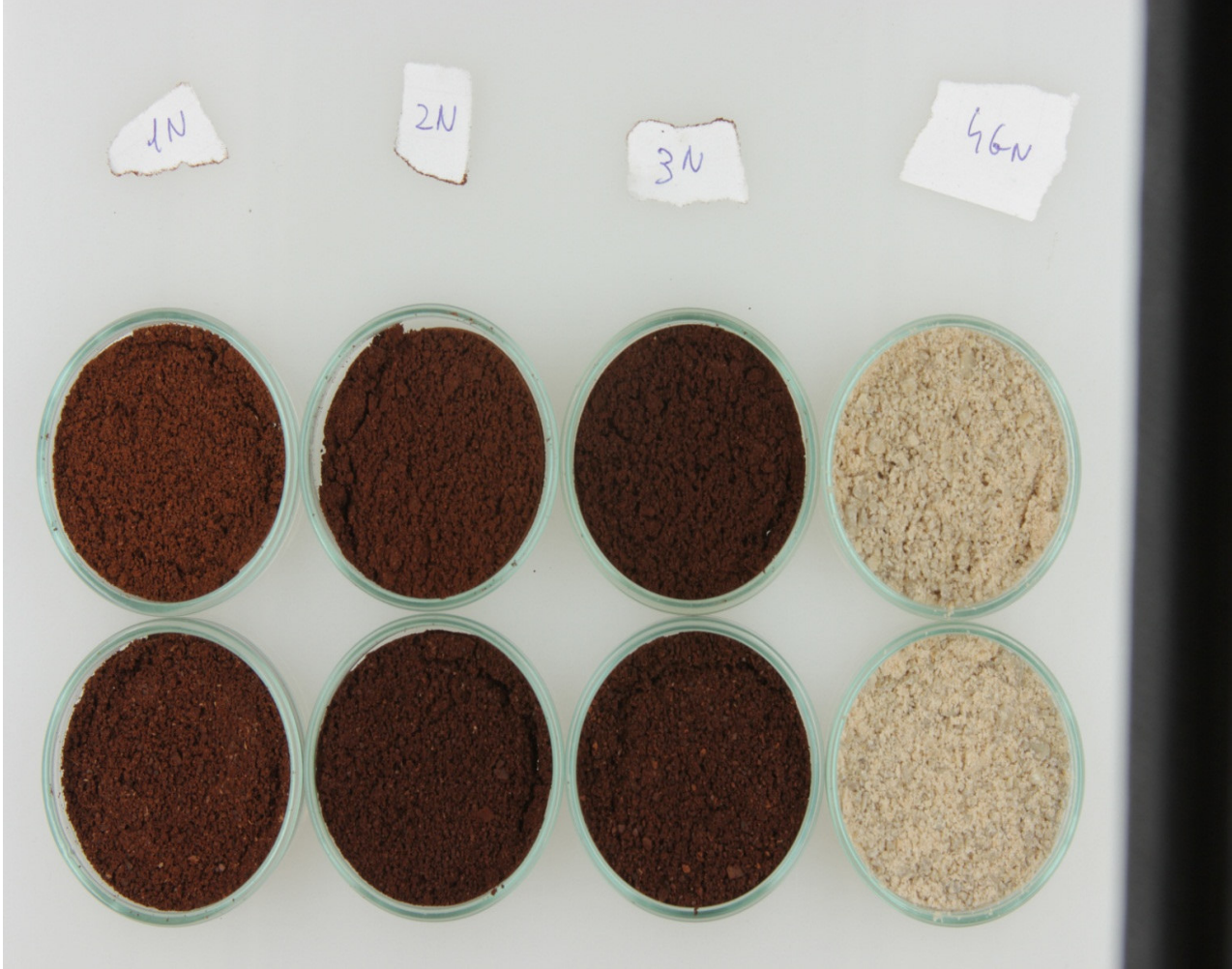
Fig. 6 Samples brewed and taken pictures. Ready for L^*a^*b^* color space measurements.
