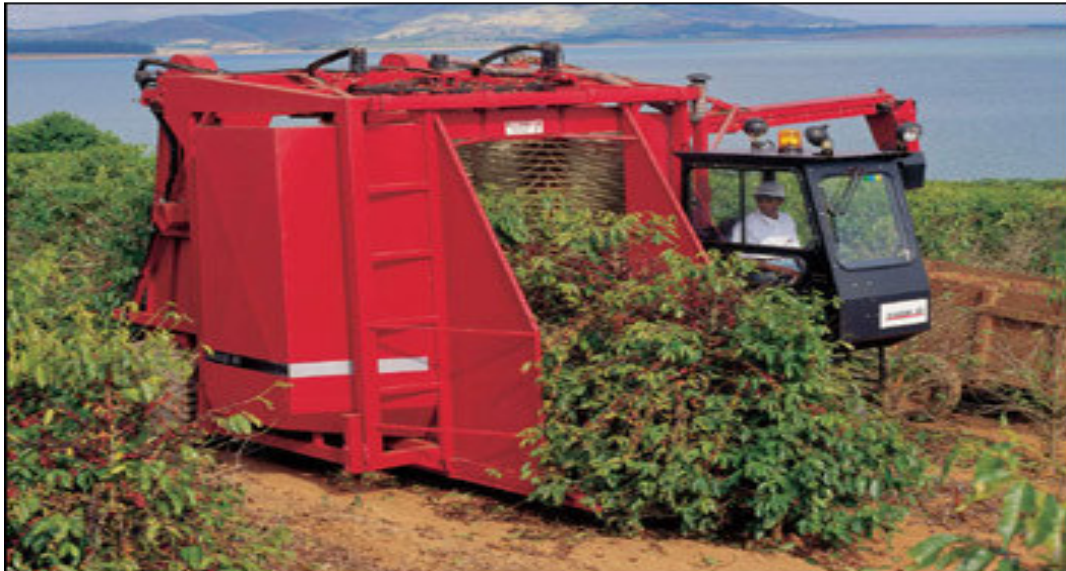
Fig. 2 Tractor – driven coffee harvesters , mainly used in Brazil and Colombia
