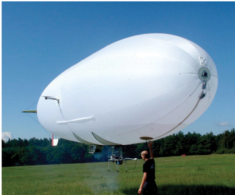
Figure 4.1: The autonomous mapping airship – AMA.
