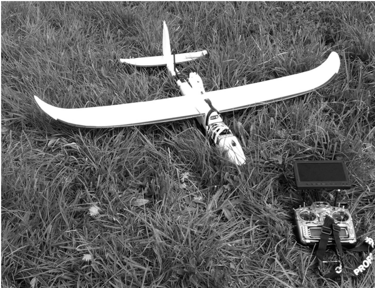
Figure 4.2: Easy Star II (wingspan 1366 mm) with 3DR Pixhawk B autopilot in the measurement locality.
