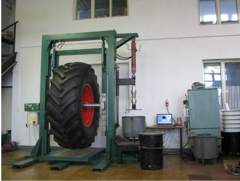
Figure 3: Laboratory equipment includes soil compactor and tyre footprint attachment; (source: author).
