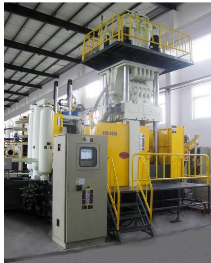
Obr. 2-12 Pohled na sekci strojů pro metodu squeeze casting (SCV Series Vertical Squeeze Casting Machine, firma Sanji) [22]
