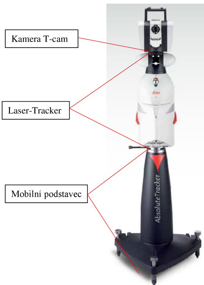
Obr. 13) Sestava 3D Laser-Tracker [14]
