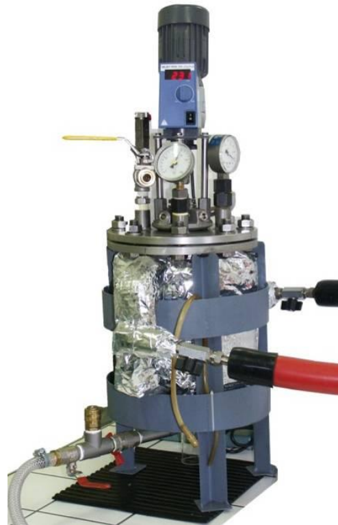
Figure 36 Disintegration unit used in experiments
