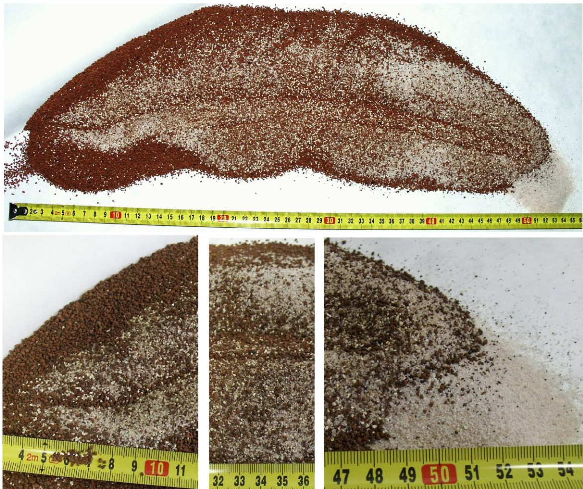
Figure 24 Material distribution in the ash collector
