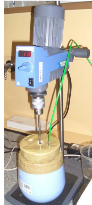
Figure 15 Experimental setup for heat capacity measurement
