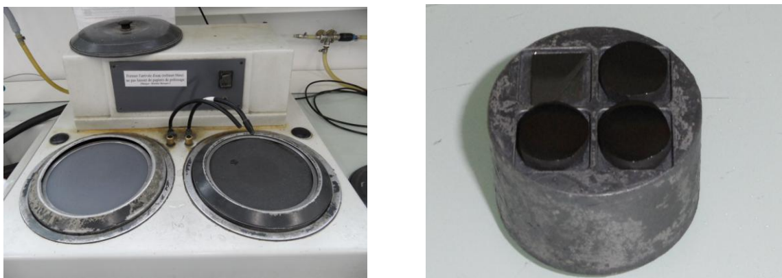
Fig. 41 Machines for polishing the substrates (left) and susceptor with substrates (right)
