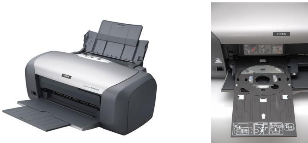
Fig. 31 Used inkjet printing Epson R220 with modified CD holder
