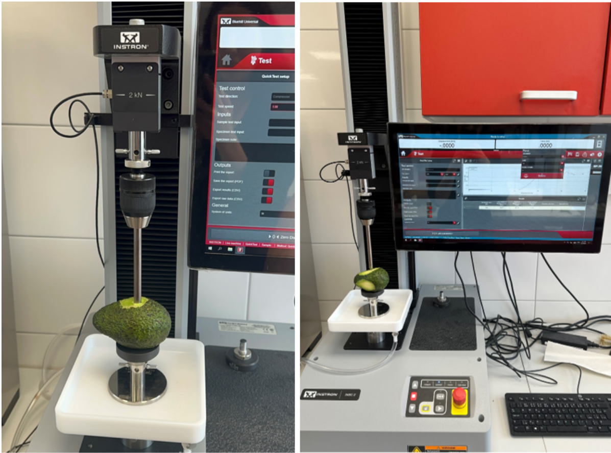
Figure 25. Measurement of the firmness of avocado on Instron penetrometer.
