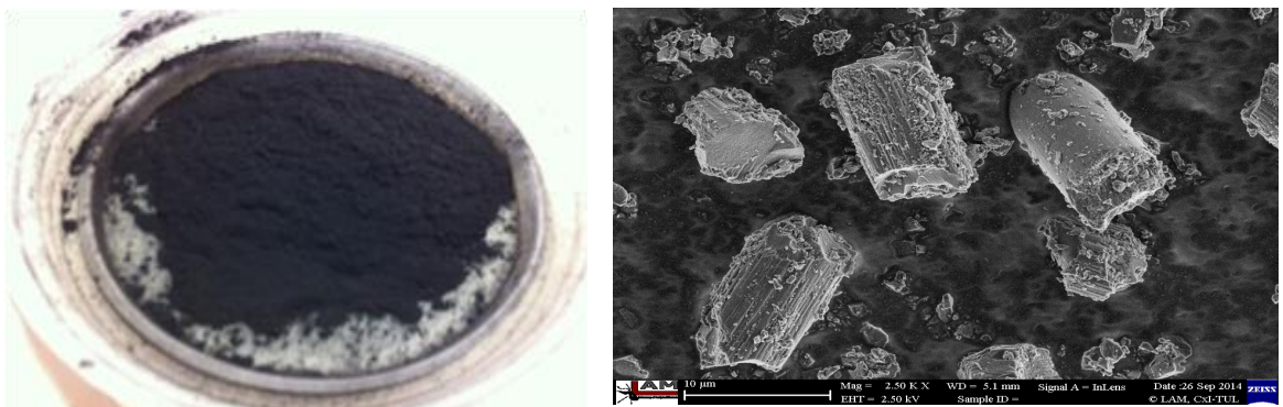
Figure 3.5 Photo and SEM of submicro carbon fibers (milled fibers)
