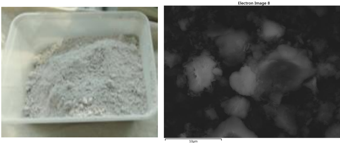
Figure 3.2 Photo and SEM picture of powder baucis L160 geopolymers
