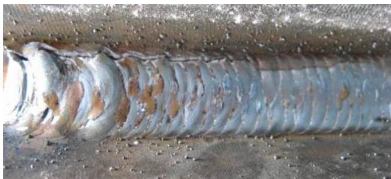
Obr. 2 - Vada studená trhlina [2]
