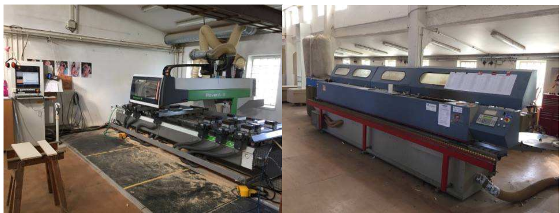
Fig. 3: a-b: CNC Biesse ROVER A 1332 5-AXIS and Edge banding machine OTT (Marek Šulc, 2017)
