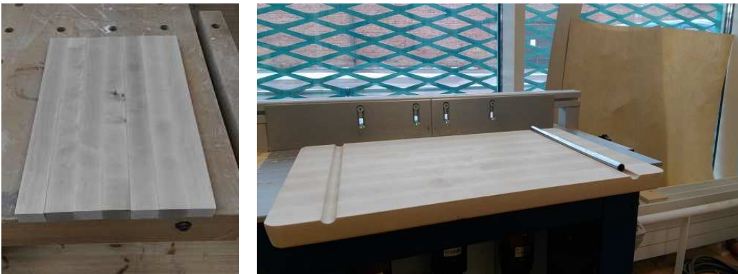
Fig. 20: (a-b): Glued board and trenched slots for tubes (author, 2016)
