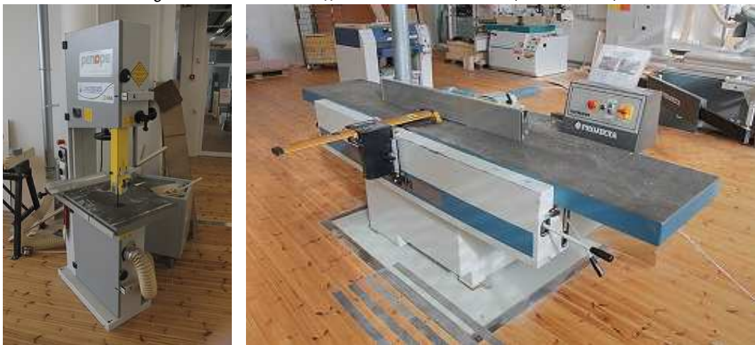
Fig. 30: a-b: Vertical Saw Penope and Surface planer Hofmann AHW 512 (author, 2016)
