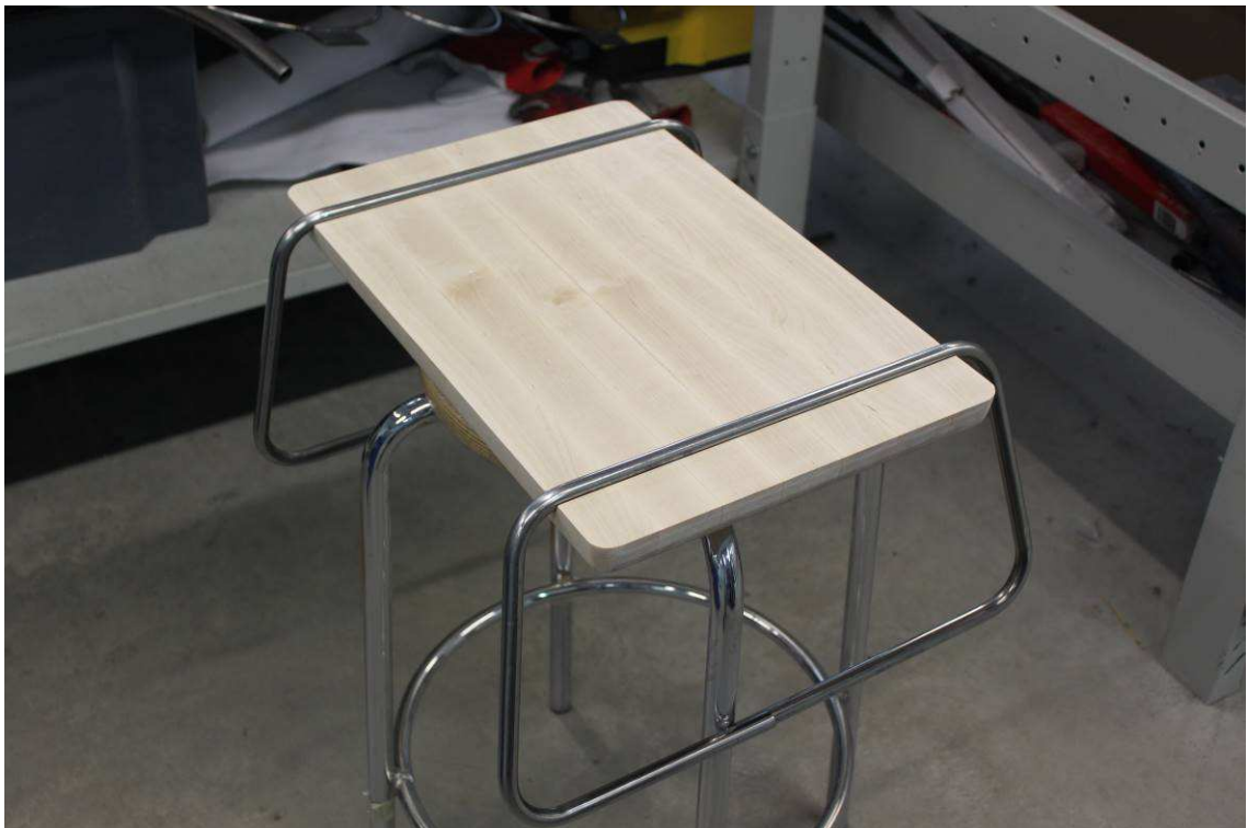
Fig. 22: Bended tubes without welded joint (author, 2016)
