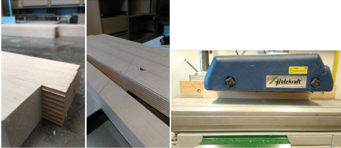
Fig. 47: a-c: Finger joint, battenboard, milling machine Holzkraft (author, 2017)
