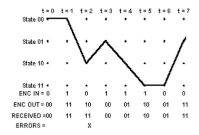
Fig. 3.8: Example of Viterbi decoder decoding process [6]
