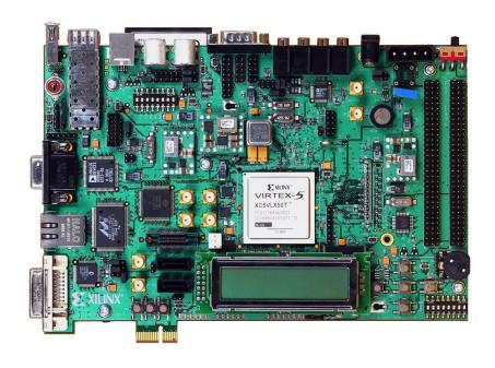
Fig. 4.2: ML505 Development Board, top view
