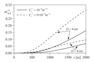
Fig. 2.5: Aperture averaged scintillation index as function of channel distance ( $\hat{r} = 1$ ,  $\rho_S = 100$ ,  $\lambda = 1.55 \,\mu\text{m}$ ,  $w_0 = 2.5 \,\text{cm}$ ) [10]
