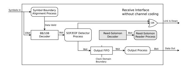
Fig. 5.13: Receive unit of the MAC, channel coding off
