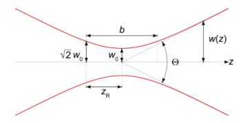
Fig. 2.1: Gaussian beam parameters [21]
