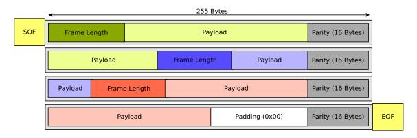
Fig. 5.9: Super-frame, output of the channel encoder with the SOF and the EOF
