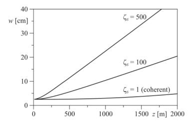
Fig. 2.3: Collimated beam size as a function of range for several choices of phase diffuser ( $\lambda = 0.785 \, \mu \text{m}$ ,  $w_0 = 2.5 \, \text{cm}$  and  $C_n^2 = 10^- 14 \, \text{m}^{-2/3}$ )[10]
