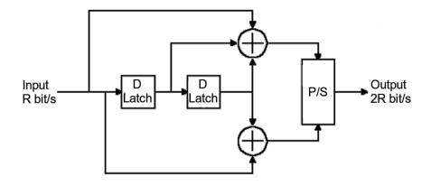
Fig. 3.7: Example of convolutional encoder with k = 1/2
