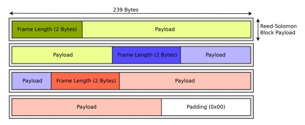
Fig. 5.8: Data input to the channel coder, three frames
