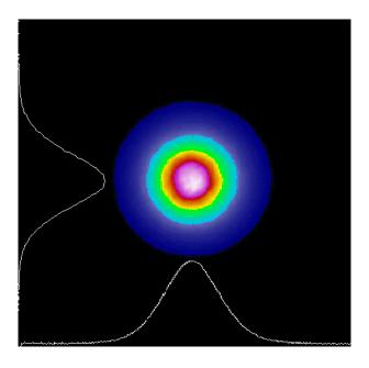
Fig. 2.2: Gaussian beam spot measured by a detector [16]
