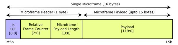
Fig. 5.18: Microframe structure
