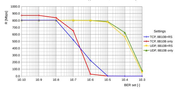
Fig. 6.11: Bit Rate In Function of Bit Error Rate of The Link
