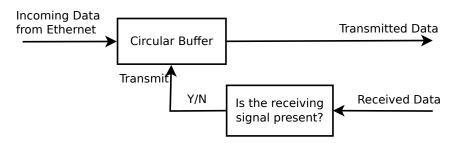
Fig. 3.10: Proposed BER/FER reduction method illustration
