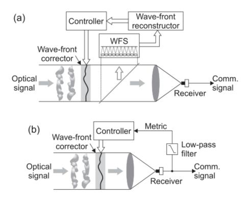
Fig. 3.3: Schematics of adaptive optics approaches for FSO communication. (a) Conventional adaptive optics uses a wave-front sensor (WFS) and wave-front reconstruction for control of the wave-front corrector. (b) Wave-front distortion compensation based on blind optimization of a system performance metric may use the received signal strength (determined from the communication signal after low-pass filtering) for the feedback [25]
