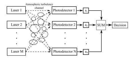
Fig. 3.1: Block diagram of M  $\times$  N MIMO FSO system over atmospheric turbulence channel [3]
