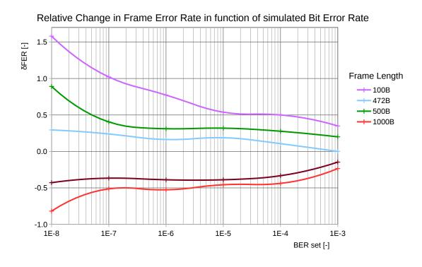
Fig. 6.10: FER Evolution After Enabling the RS Coder,  $\delta FER$  defined in 6.2
