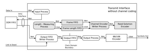
Fig. 5.6: Transmit unit of the MAC, channel coding off
