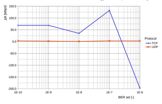
Fig. 6.12: Difference of Bit Rates In Function of Bit Error Rate
