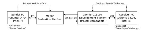
Fig. 6.8: Experimental Setup for BER Measurements
