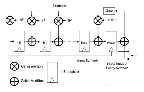
Fig. 3.5: Block diagram of RS encoder [19]
