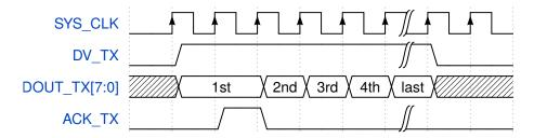
Fig. 5.5: Transmit interface, TEMAC compatible
