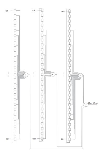
Fig. 3.9: LDPC encoder example, k=3/4 and L=108bits [18]
