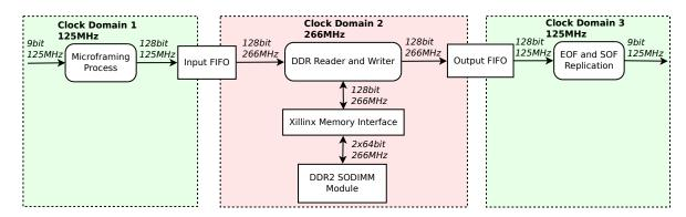
Fig. 5.17: DDR FIFO internal data flow
