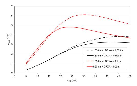
Fig. 1.1: Attenuation caused by turbulence for two values of receiver's lens diameter and for two wavelengths in function of the link range [11]
