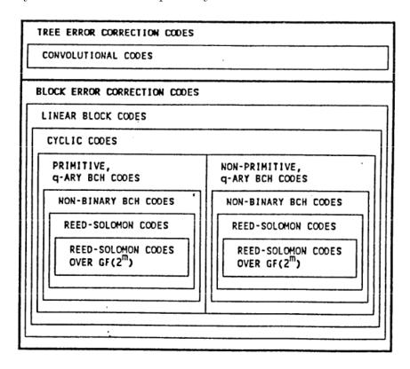
Fig. 3.4: Venn diagram to classify the RS code [5]
