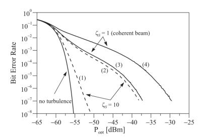
Fig. 2.6: Effect of optical turbulence on BER as a function of received optical power for collimated ( $\hat{r}=1$ ) coherent ( $\rho_S=1$ ) and partially coherent ( $\rho_S=10$ ) beams ( $\lambda=0.785~\mu\text{m},~w_0=2.5~\text{cm},~z=2000~\text{m},~D=10~\text{cm}$ ). Left to right (1)  $\rho_S=10, C_n^2=10^{-15}~\text{m}^{-2/3}$ , (2)  $\rho_S=10, C_n^2=1.210^{-14}~\text{m}^{-2/3}$ , (3)  $\rho_S=1, C_n^2=10^{-15}~\text{m}^{-2/3}$ , (4)  $\rho_S=1, C_n^2=1.210^{-14}~\text{m}^{-2/3}$  [10]
