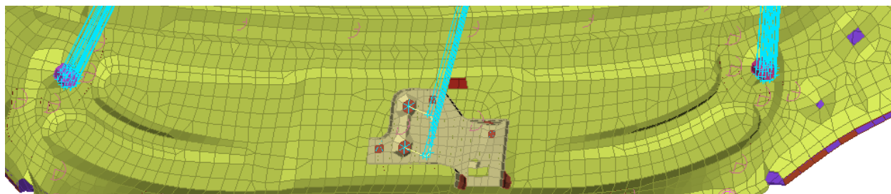
Figure 9.3: Rigid body condition to the bonnet rubber stops and front lock
