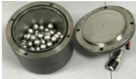
Fig. 17 Steel milling jar containing steel balls for mechanical alloying of powders fabricated in-house.
