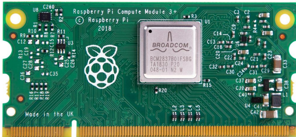
Obr. 3-14 Raspberry Pi Compute Module 3+ [44]
