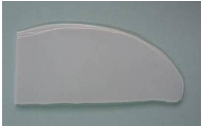
Fig. 5.14 1 mm thick UV cured sheet comprised of 4 layers.
