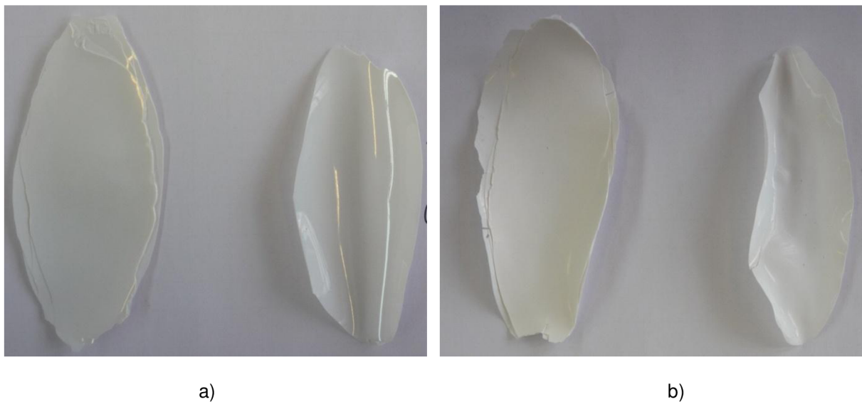
Fig. 5.30 UV cured multilayer (left) and monolayer (right) sheets of the suspensions with: a) 15 vol% of DIW substituting 15 vol% of monomer mixture and b) 30 vol% of DIW substituting 30 vol% of monomer mixture.
