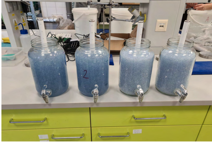
Figure 4.3: Obtaining raw signal values at artificial porous environment. Two left buckets are representing a fully saturated environment. Right buckets represent dry conditions. Glass beads of size 2mm were used to simulate the soil environment.
