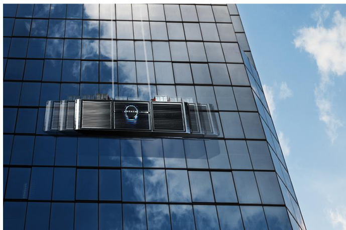
Figure 3. Façade maintaining robot Homan Printed from https://autonomia.com/homan/
