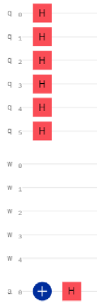
Figure 4.2: Initialisation circuit component for N = 64
