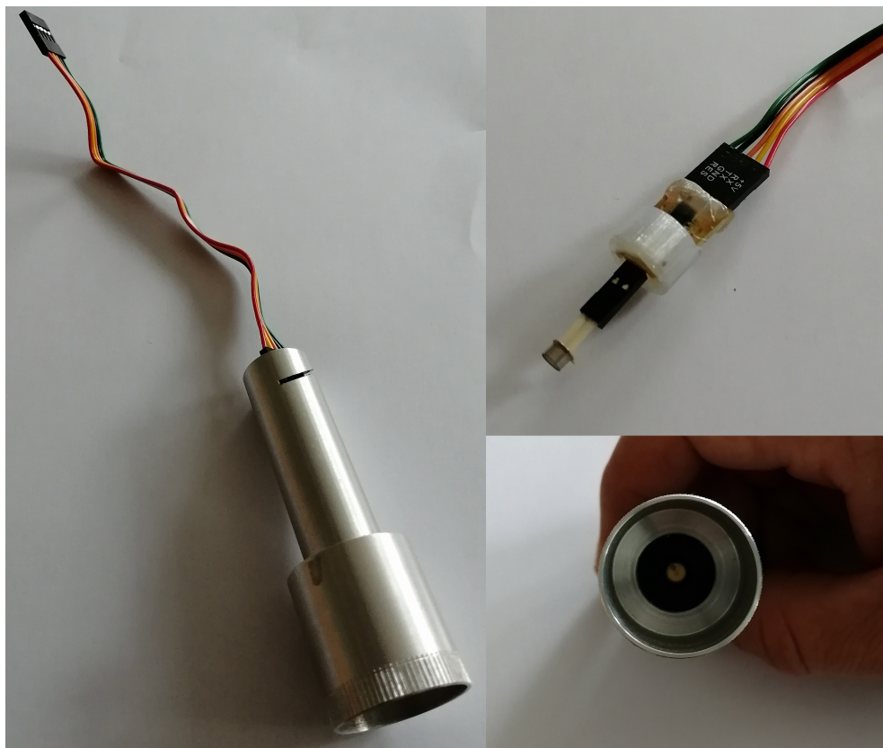
Figure 33 | Photos from various angles of the UV LED flasher used in calibration measurements.
