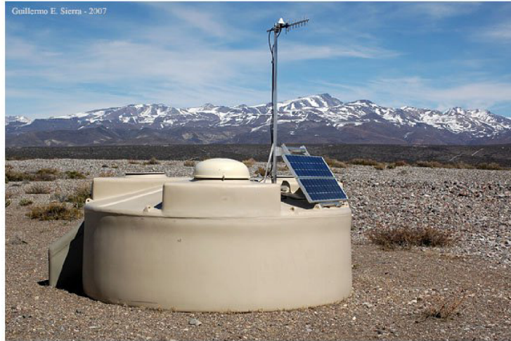
Figure 6 | An image of a surface detector in Pierre Auger Observatory in Argentina. [8]
