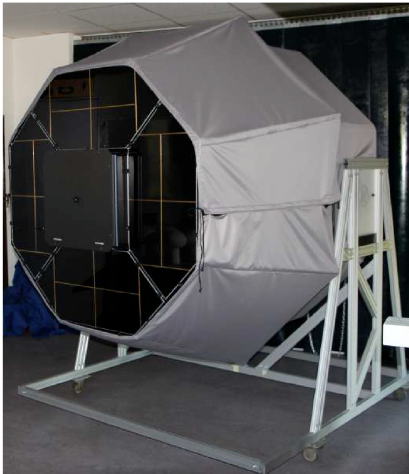
Figure 17 | An image of the FAST telescope, including the aluminum structure, octagonal UV filter and a protective shroud. [11]
