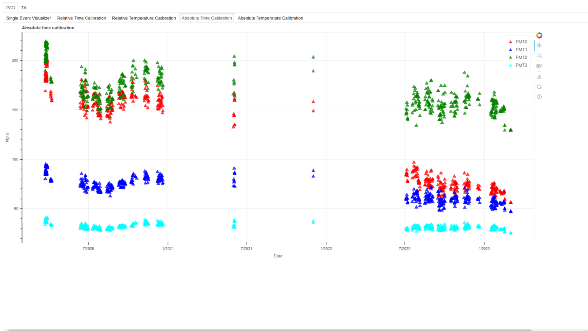
Figure 64 | Absolute temperature calibration of PMTs demonstrating low gain on the FAST telescopes located on the TA site.
