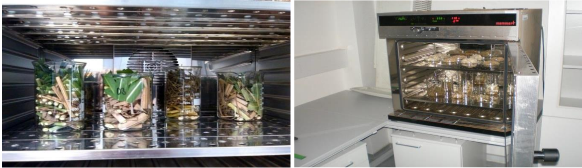
Figure 11: Samples in laboratory oven MEMMERT model 100-800 Source: Medová (2015)
