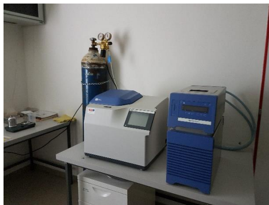
Figure 12: Calorimeter IKA C6000 Source: Author
