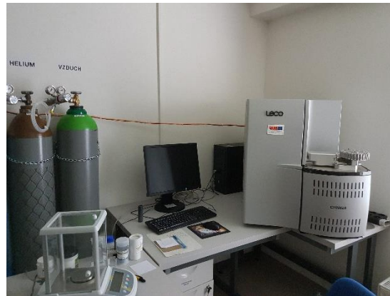
Figure 13: Elementary Analyser LECO CHN628 Source: Author
