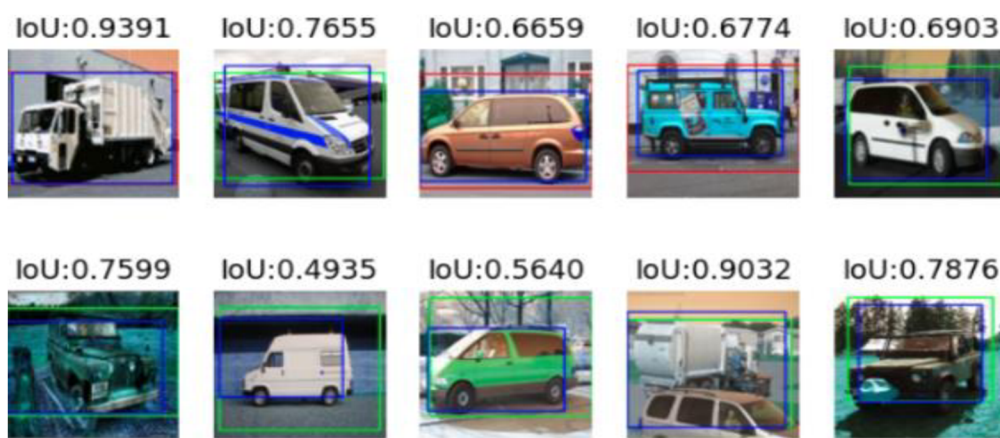
Figure 4.13 Visualization of bounding boxes with different colors (blue: ground truth, green: predicted box with true label, red: predicted box with false label)
