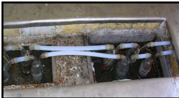
Figure 9.6 Condensation of tar during sampling
