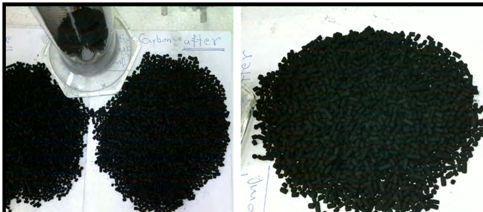
Figure 12.14 Active carbon material pre and posts multiple uses in the experiments
