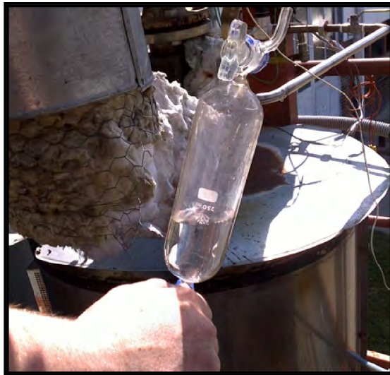
Figure.9.13 Gas sampling post filter
