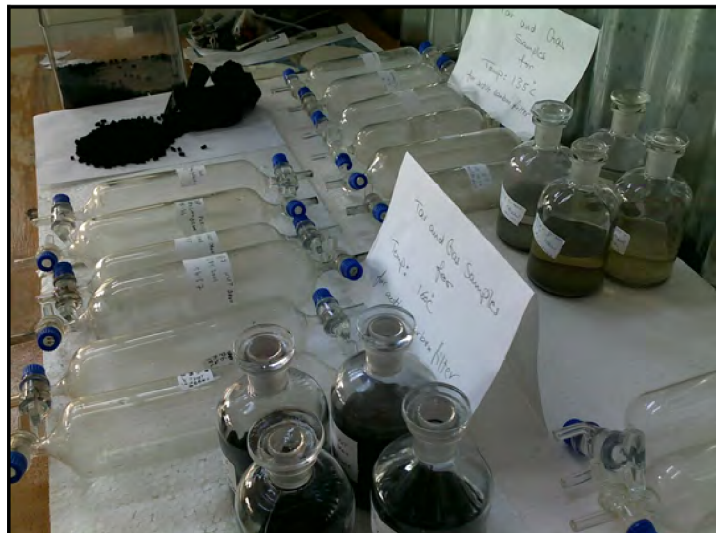
Figure.9.15 Final gas and tar samples
