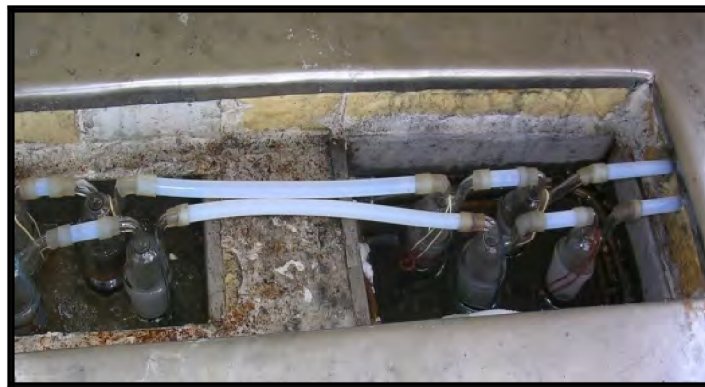
Figure 9.6 Condensation of tar during sampling
