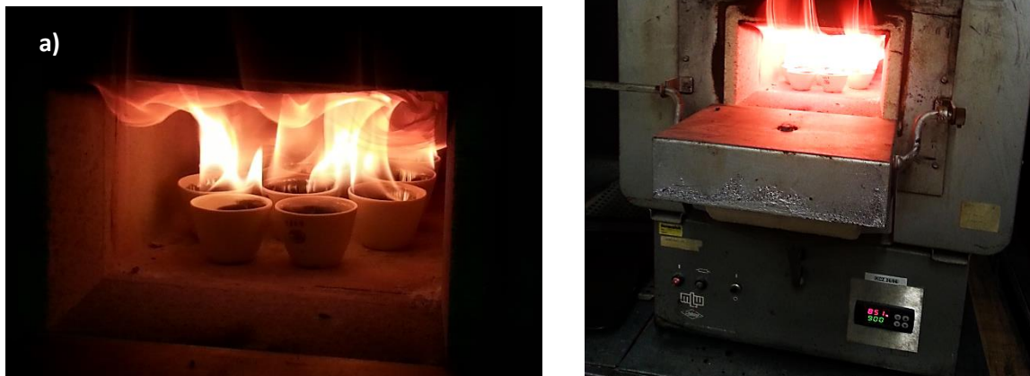
Figure 5. Determination of ash. (a) Porcelain dish with composite flour which carbonized by flame; b) muffle furnace).
