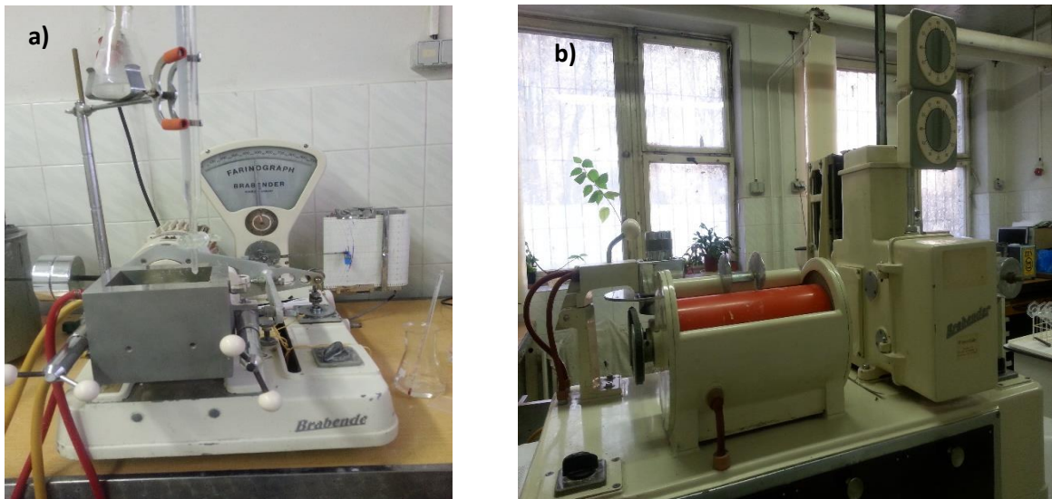
Figure 4. Rheological methods equipment: a) Farinograph; b) Extensograph
