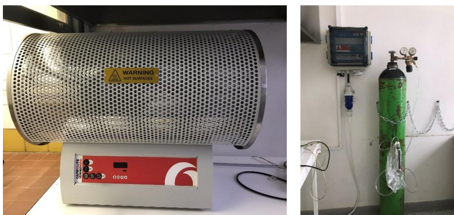
Figure 8 Furnace Carbolite® Typ 301 and Nitrogen source
