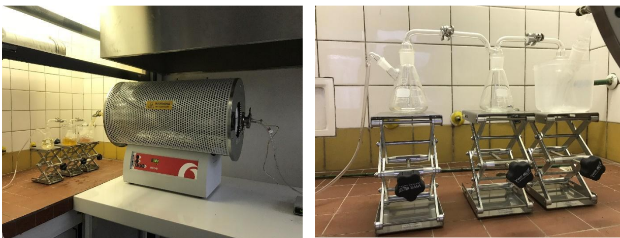
Figure 10 Volatiles collecting setting
