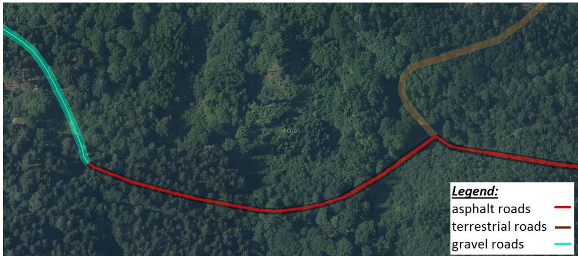
Figure no.13: Detail of FR areas accoring to different types of surface
