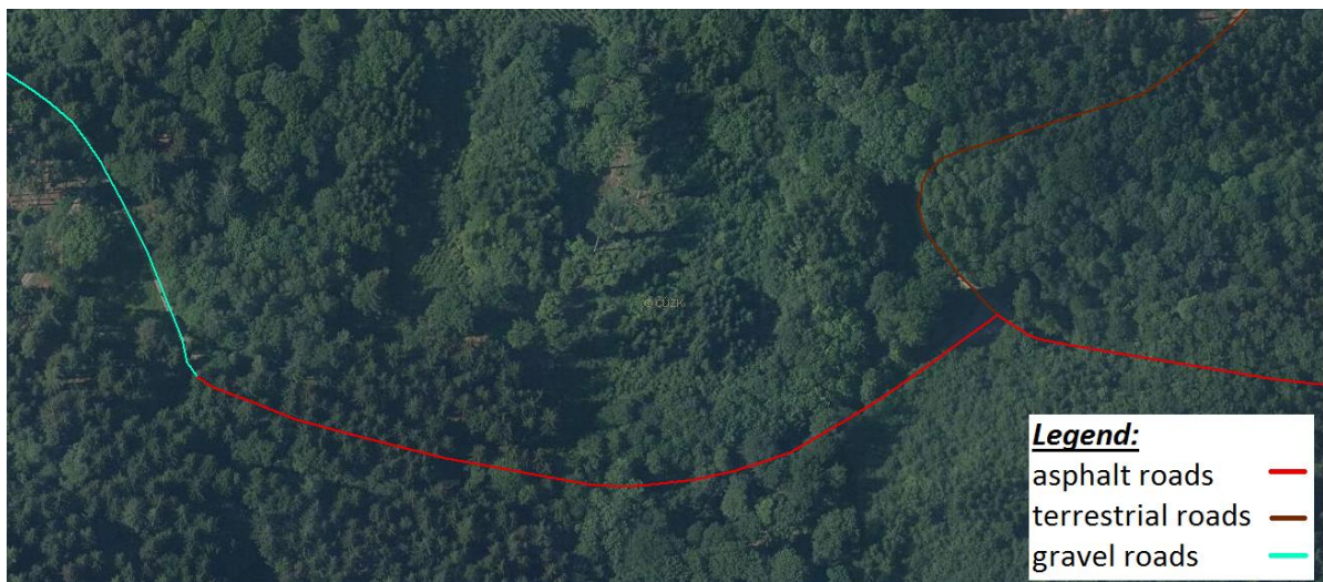
Figure no.12: Detail of axis of FR according to different types of surface
