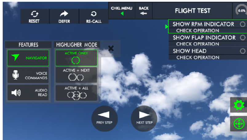
Figure 6.9: Top panel displays progress indicator, title, step back button, and drop down checklist menu. The checklist menu differs with respect to the displayed list. The reset button is displayed always. If a checklist is displayed on the task panel, the checklist menu contains defer and recall buttons.
