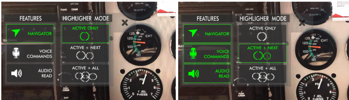
Figure 6.14: Setting panel allows to enable or disable implemented features and change highlighter mode.
