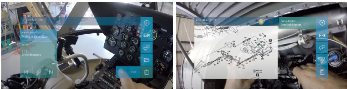
Figure 3.4: Atheer's AiR Enterprise is used to inspect a helicopter 6 .
