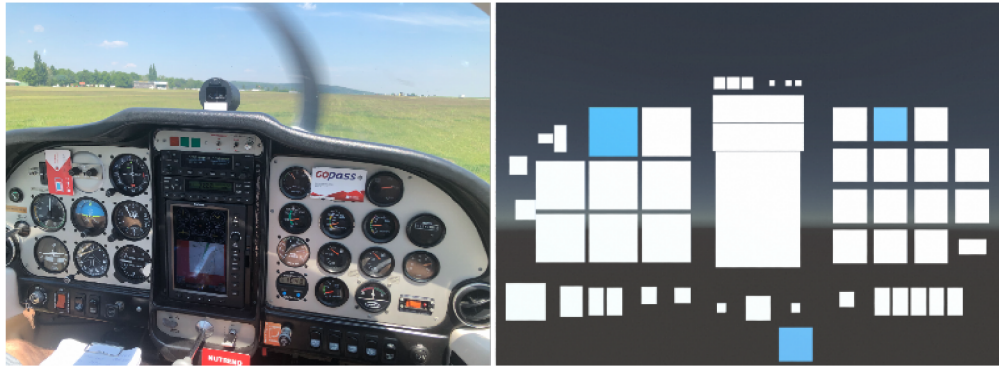
Figure 7.2: Comparison of flight deck on the left side and virtual 3D model on the right side. Model elements marked blue represents an image markers.
