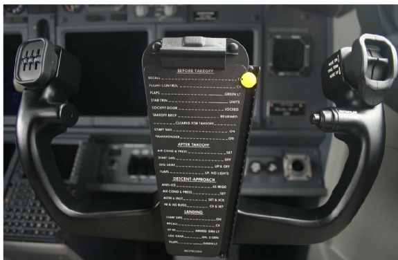
Figure 3.8: Checklist attached to yoke in Boeing 737 10 .
