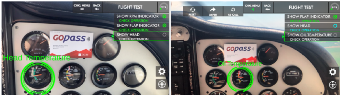
Figure 6.11: Left: Flight instrument marking in the default mode. Right: An active step can be deferred through Defer button.
