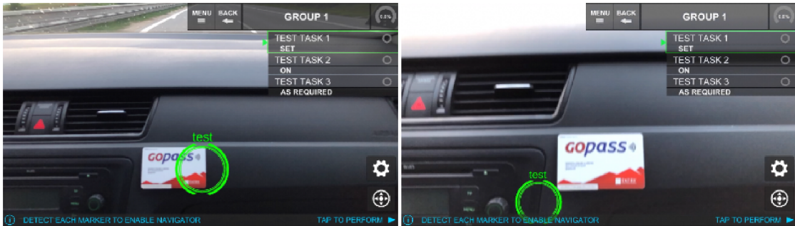
Figure 6.7: Left: Required state. Right: The system has lost tracking ability.
