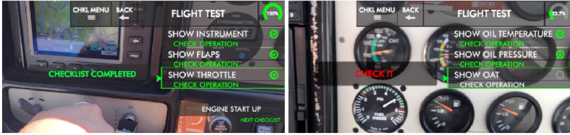
Figure 6.13: Left: Message indicating completion of the checklist. Right: Active task was confirmed but flight instrument was not even in the field of view.
