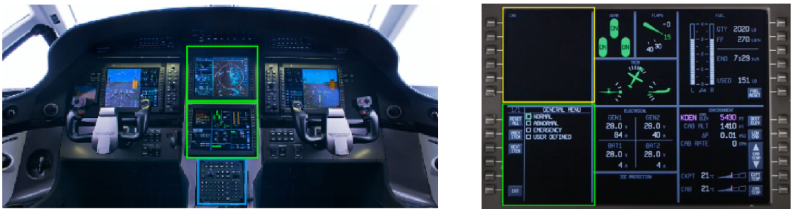
Figure 4.7: Left: PC-12 cockpit flight deck 9 . Right: System MFD display layout 10 .
