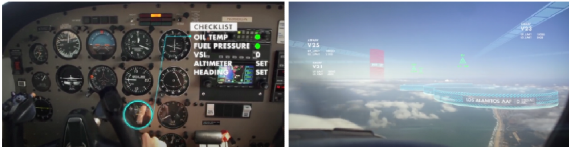
Figure 3.5: Aero Glass presented concept of AR in cockpit 7 .
