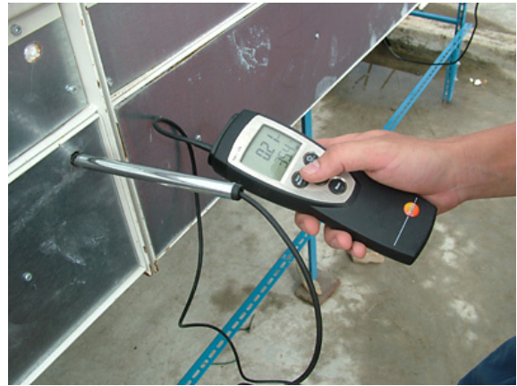
Fig.3.6. Measuring the air-flow in the drying chamber.
