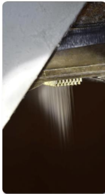
Figure 9: Formation of fibers on the Spun-blown machine
