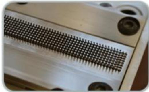
Figure 8: Spinneret of the spun blown machine
