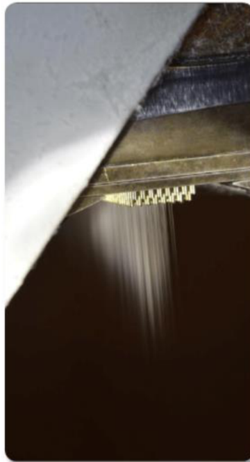
Figure 9: Formation of fibers on the Spun-blown machine
