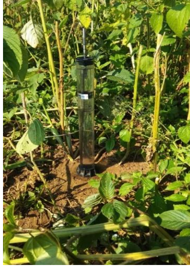
Figure 17 Measurement of unsaturated hydraulic conductivity with Mini Disk Infiltrometer (Source War War Mon)
