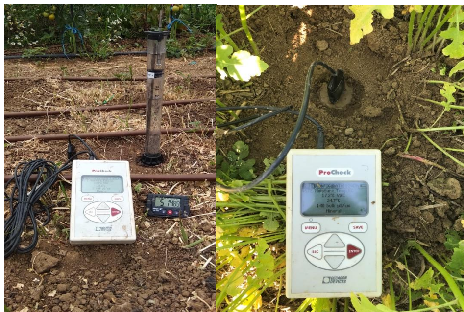
Figure 18 Measurement of water content with 5TE sensor (Source War War Mon)
