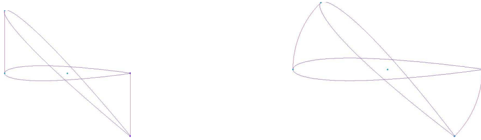
Figure 6.2: Rotation of the airfoil prescribed through linear mode shapes (left) and through rotational matrix (right)
