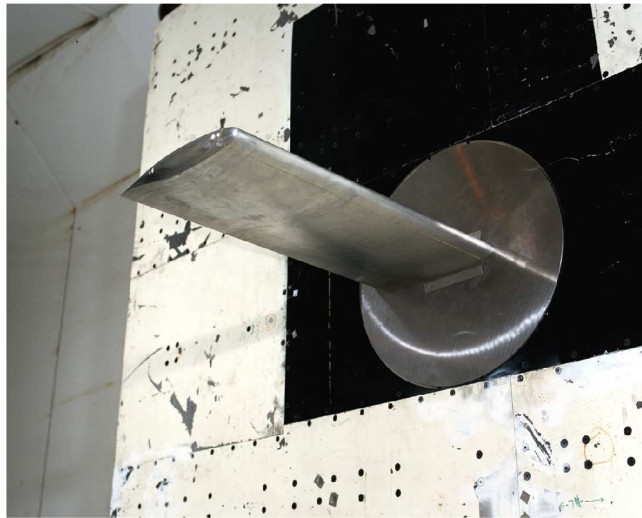
Figure 6.3: BSCW wing at NASA TDT wind tunnel section, Courtesy of NASA
