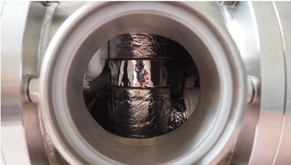
Figure 33: Specimens with shielding in test chamber.
