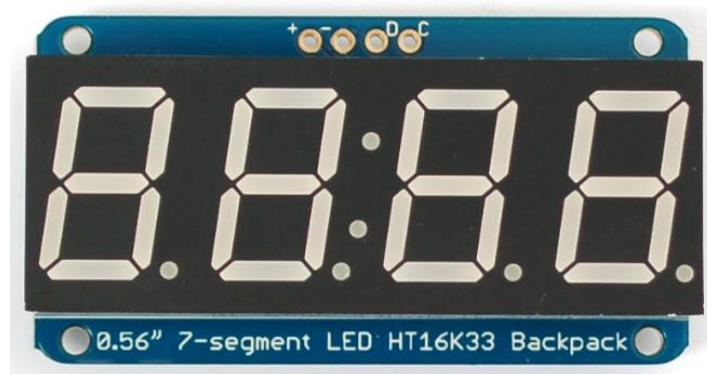
Obrázek 7 - 7 - segment LED HT16K33 Backpack [9]
