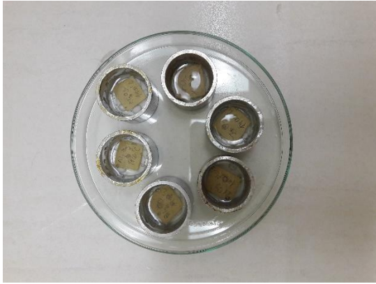
Fig. 16: Labeled molds after mounting
