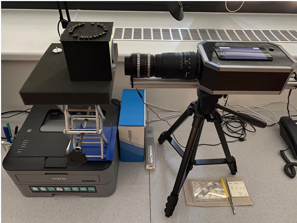
Fig. 18: Experimental equipment for sessile-drop method
