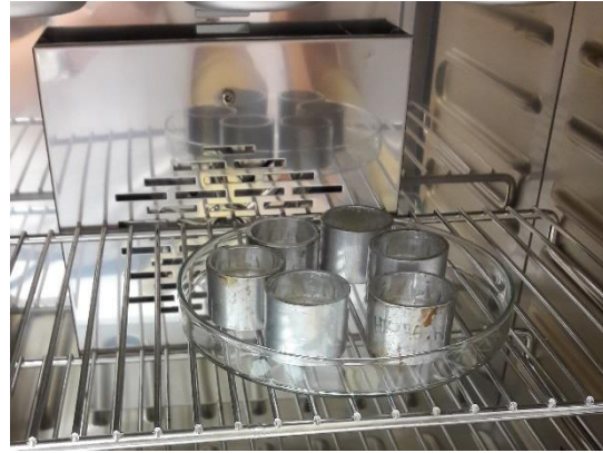
Fig. 17: Mounting in the heating oven
