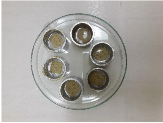
Fig. 16: Labeled molds after mounting
