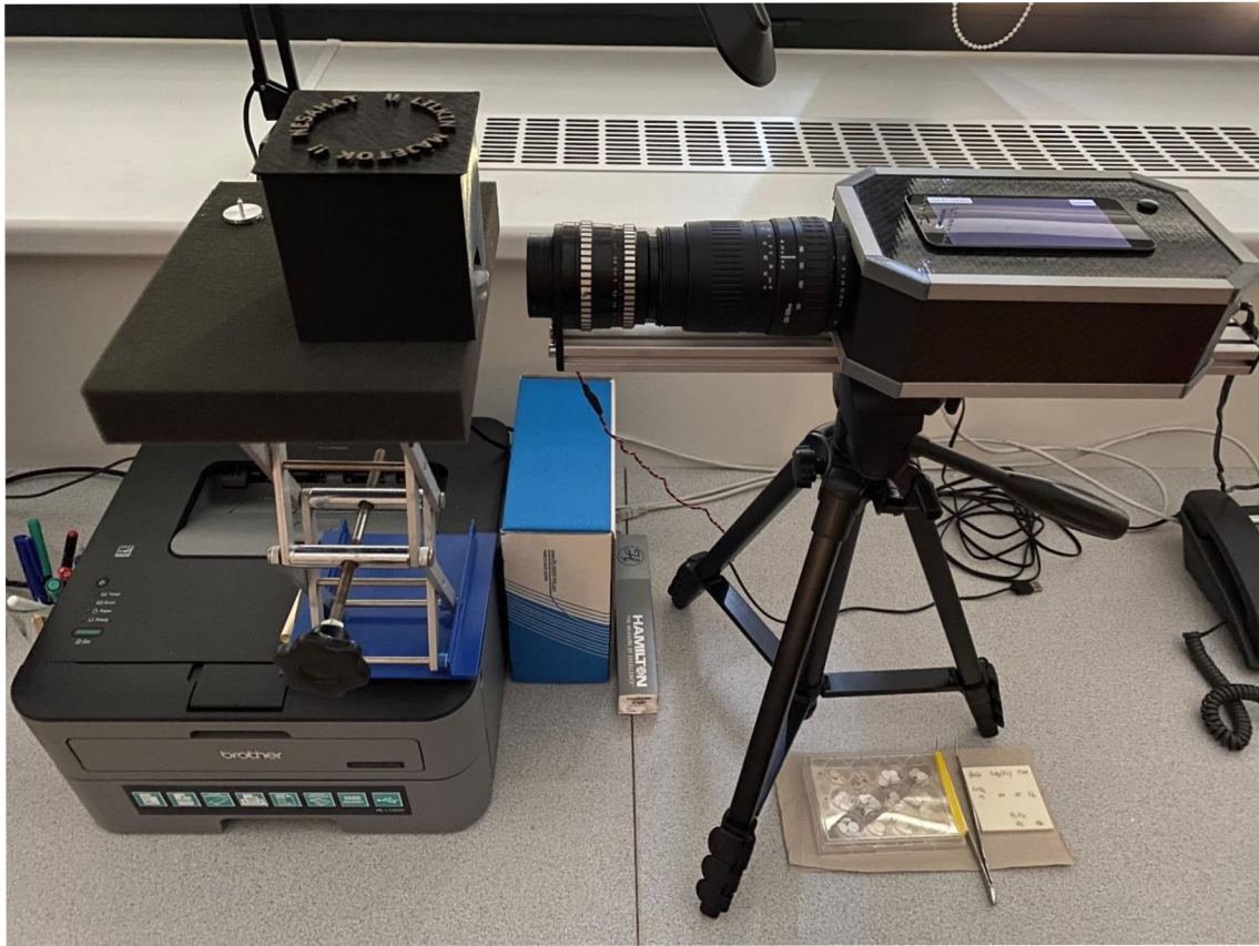
Fig. 18: Experimental equipment for sessile-drop method
