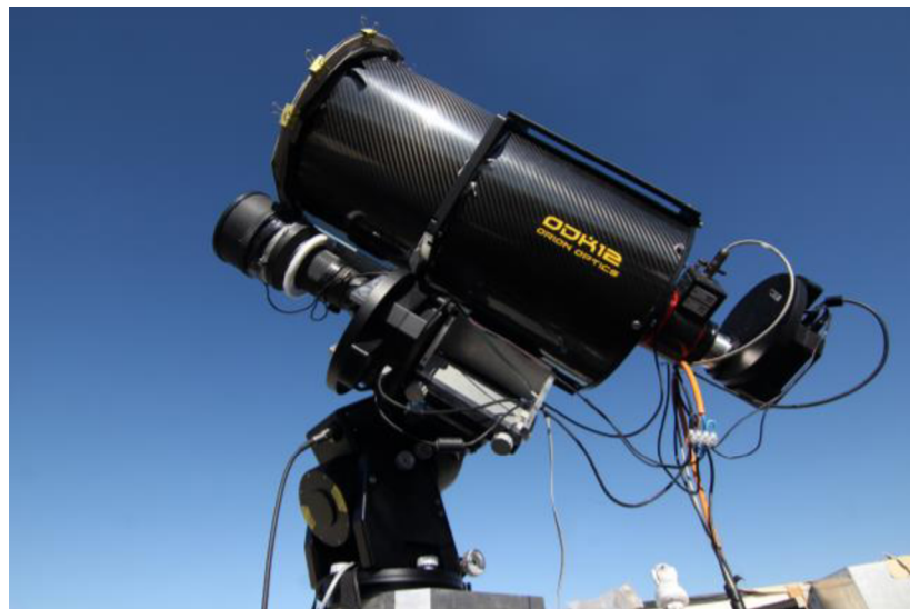
Figure 5: The current set-up of the FRAM telescope where the narrow-field system is on the top and the wide-field system is on the bottom. [19]
