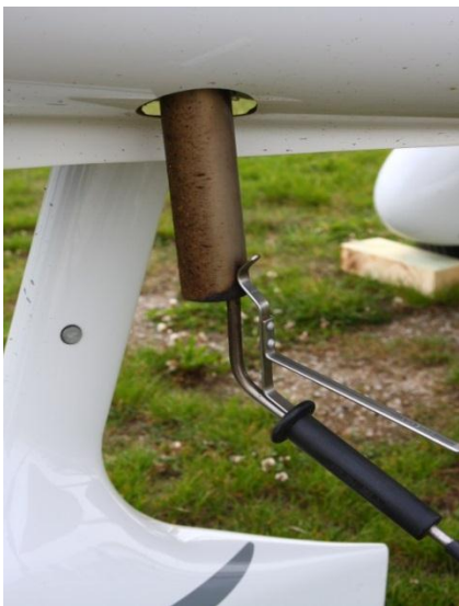
Fig 11 Sensor connected to the exhaust pipe
