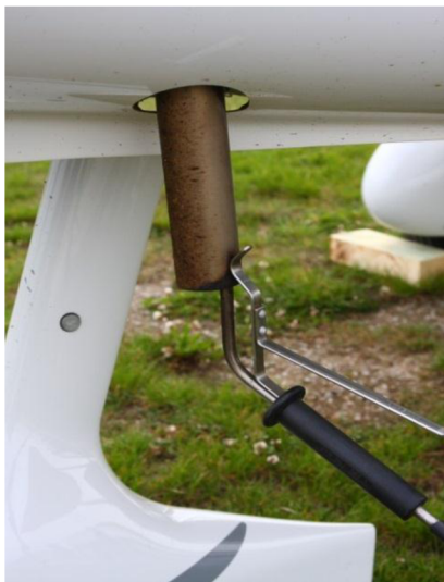
Fig 11 Sensor connected to the exhaust pipe
