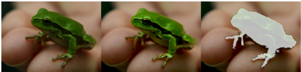
Figure 19: Brightness altering of an image part. a - Original. b - Multiplying luminance. c - Adding luminance. The scale is calculated for observing via display / prints with gamma correction 2.2
